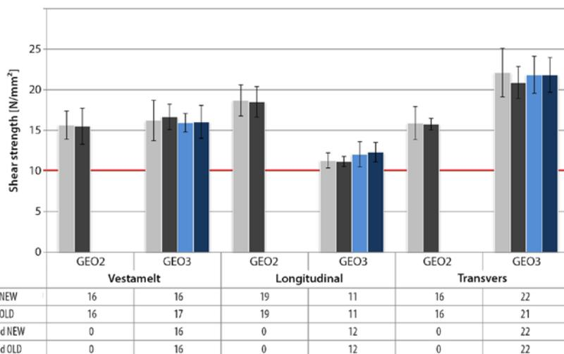
Figure 11 Shear strengths of aluminium pipes subject to various structuring compared to the serial-produced “Vestamelt” at GEO2 and GEO3 positions (© Daimler)
