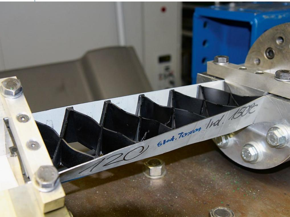
Figure 7 Structure of the torsion test for the Berlin test beam, where the failure of the ribbed section can be clearly seen (© inpro)
