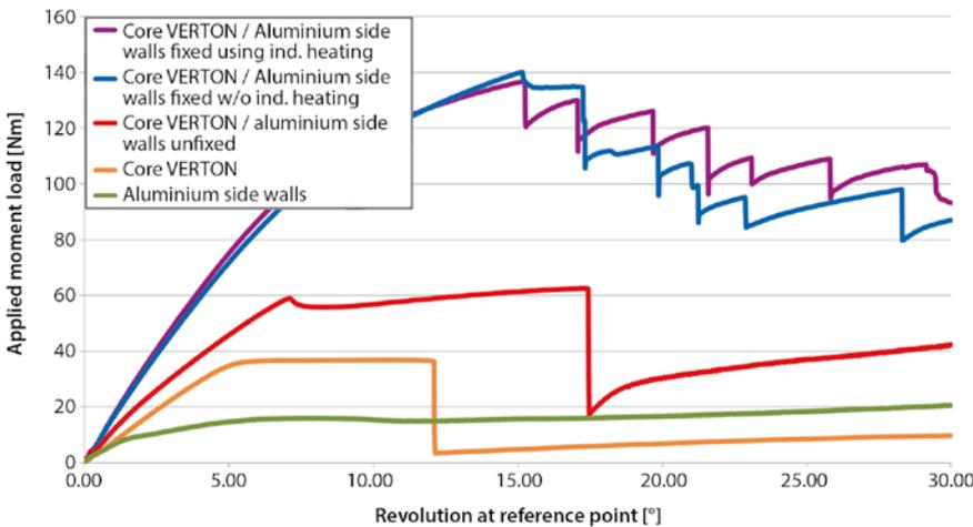
Figure 8 Torsional results for the individual components and the overall Berlin test beam (© inpro)
