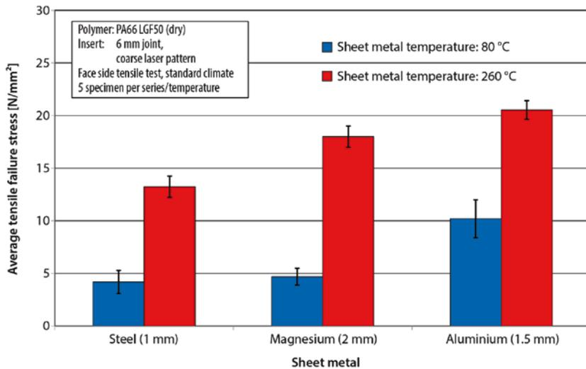
Figure 5 Impact of sheet pre-heating on steel, magnesium, aluminium (© NMF)
