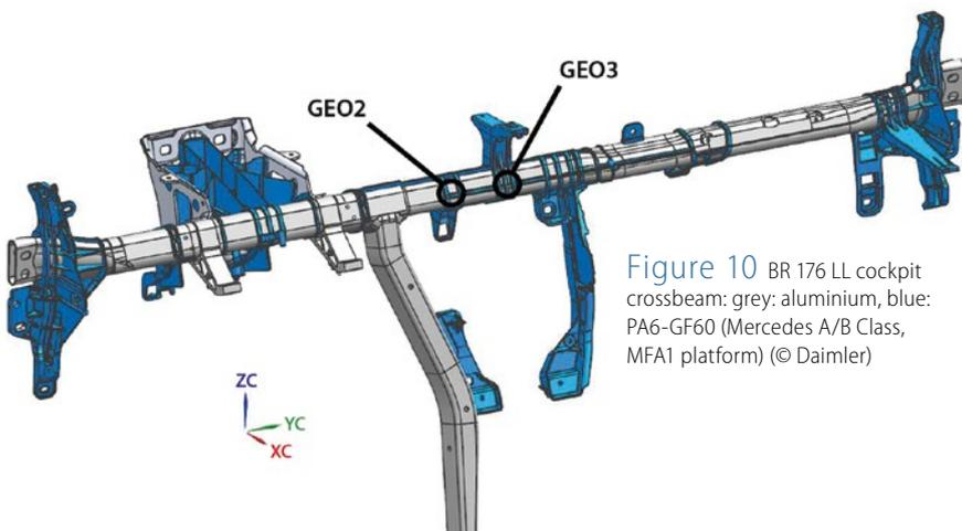
Figure 10 BR 176 LL cockpit crossbeam: grey: aluminium, blue: PA6-GF60 (Mercedes A/B Class, MFA1 platform) (© Daimler)
