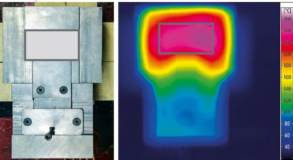
Figure 3 Temperature distribution in the middle cavity during induction heating (© NMF)
