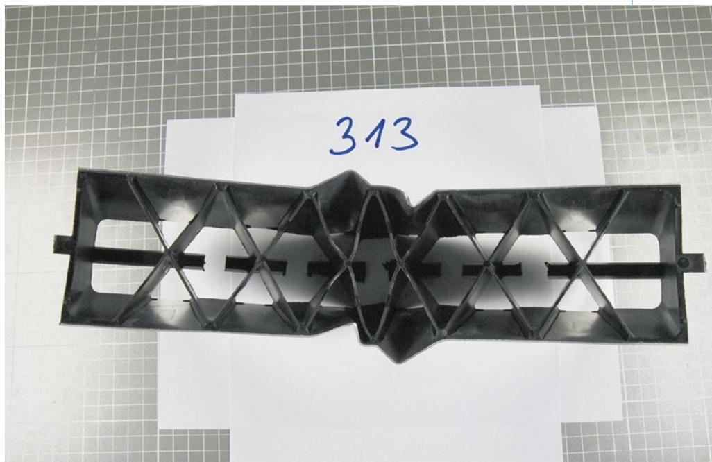
Figure 9 Berlin test beam after the bending test: The folded external sheets are clearly visible; the plastic follows in such a manner that the bond remains intact (© inpro)
