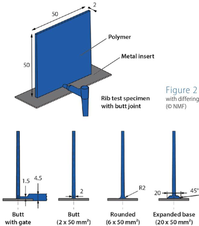
Figure 2 Ribbed test items with differing connection geometries (© NMF)
