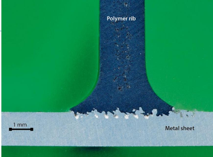
Figure 4 Transverse microsection through a ribbed test body (PA6-GF30/aluminium, rough structuring) (© NMF)
