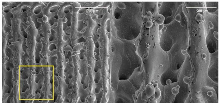
Figure 1 Laser-structured steel surface (© TRUMPF)
