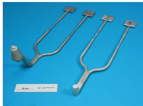
Figure 7: Different runner systems for tensile bars in thixomolding: conventional runner (left side) and hot runner (right side)
