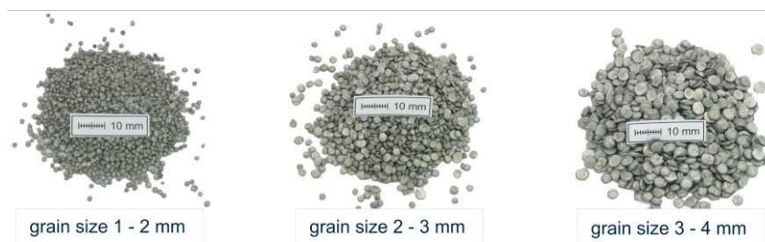
Figure 14: Different grain sizes of granules produced by a melt metallurgical process at NMF.
