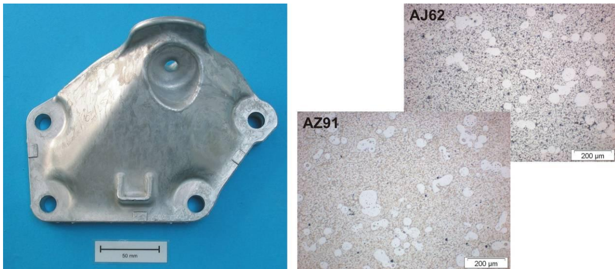
Figure 3: Engine bracket produced at NMF using Thixomolding (left) and examples for the microstructure.
