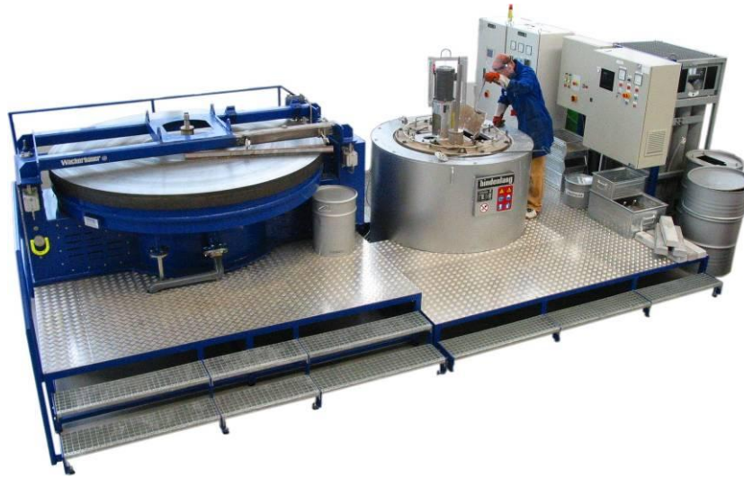
Figure 13: Equipment for the melt metallurgical production of Magnesium granules at NMF.
